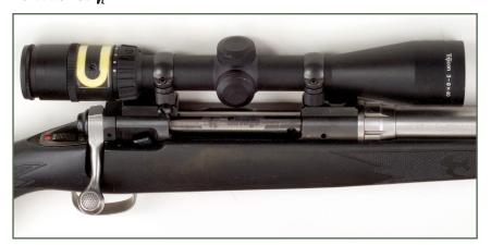
The fiber-optic collector bundle on the top of the ocular powers the triangular aiming point by gathering available ambient light. A cover allows the user to reduce brightness. For very dark conditions, a tritium lamp powers the aiming point.
